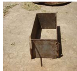
Mold made of metal sheets – Holeta Research Center
