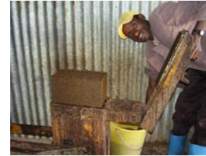
Machine for making solid construction blocks
